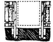
of the gate and the distance between the inside of the two gates posts to ensure the gate can swing freely. After the gate has been constructed properly for the space desired, attach the hinges and gate latch. If you desire a stop, nail a piece of fencing material to the latch post.
